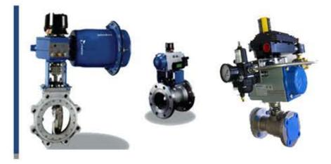
A limit switch is a valve automation accessory. They can be used with various types of actuators to remotely identify whether a valve is open or closed. The limit switch is mounted on the actuator and communicates electronically with the facility's process control system. Limit switches can help identify problems in the valve automation system before potentially dangerous and costly accidents occur.
